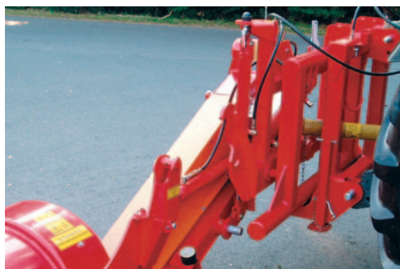
hydraulic transport protection in working position
