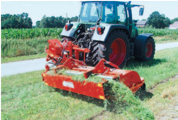
USM with conveyor belt for lateral depositing of the mowed material
