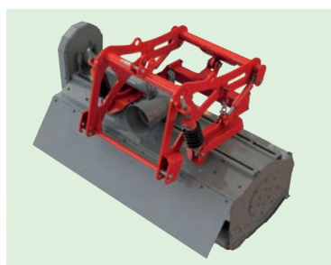
Bild 5) Front attachment pulling and guided suspended
