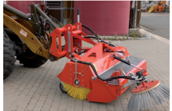
HDK on wheel loader with height compensation
