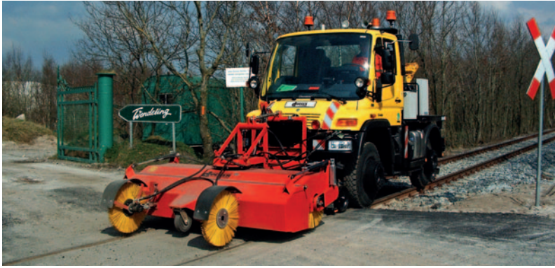
Two brushes can be installed vertically on the dirt collection bins to clean rail grooves.
