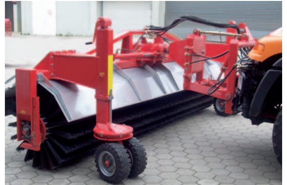
Ground adjustment via height-adjustable wheels
