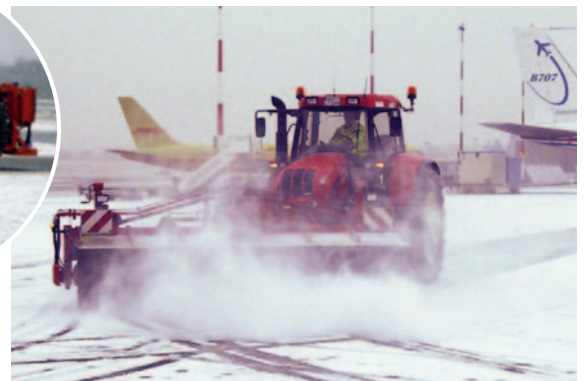
GFK on the tractor with rear-attached hydraulic unit
