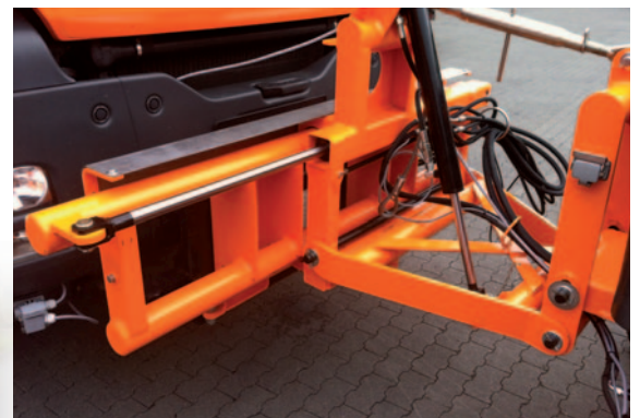
hydraulic lateral adjustment by 0.60 m
