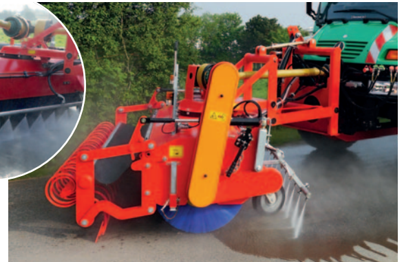
Special version of the SFK 2200 with scraper bar, high-pressure water equipment and spray bar
