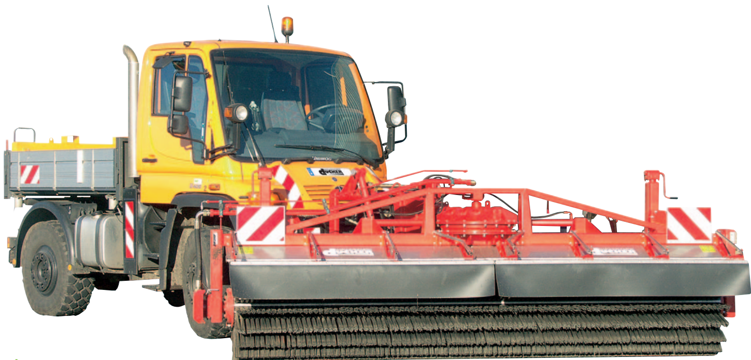
GFK on the tractor with rear-attached hydraulic unit
