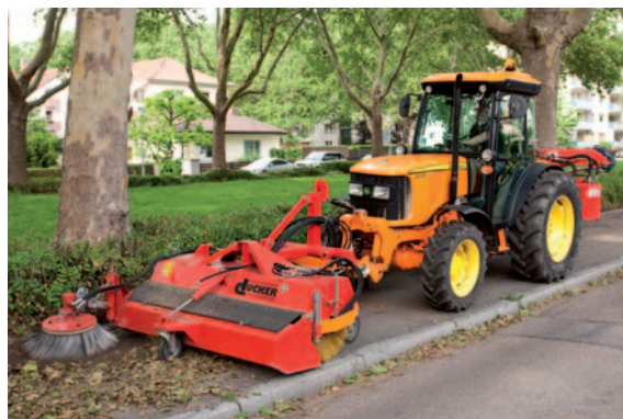
HDK with rotary side brushes in action
