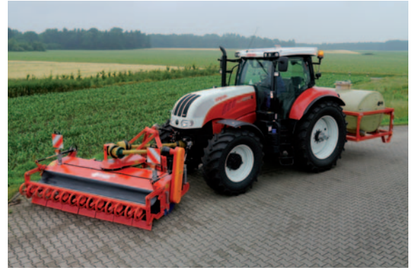
SFK with dirt scraper bar and high-pressure water equipment as rear attachment
