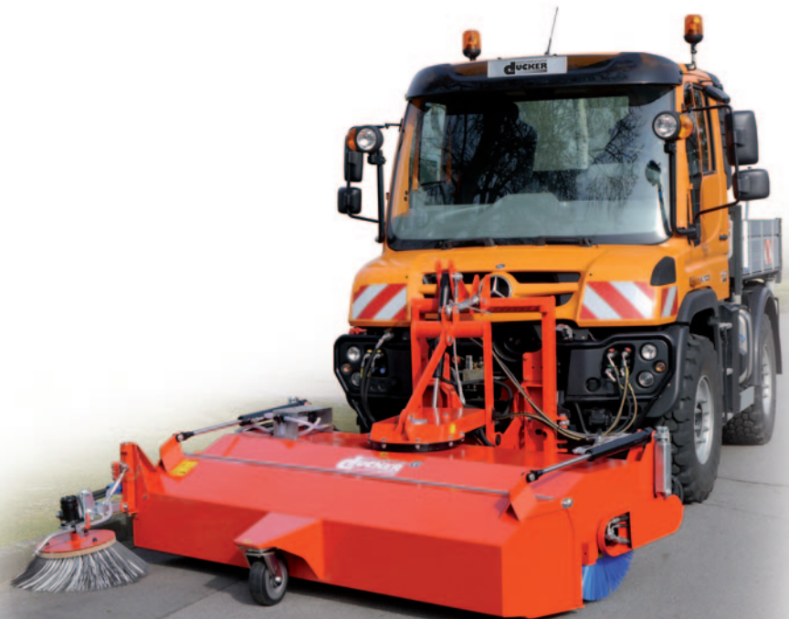
hydraulic lateral adjustment by 0.60 m
