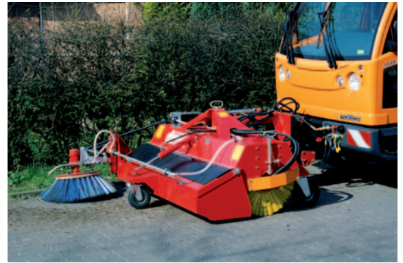
HDK with dirt collection bin and rotary side brush
