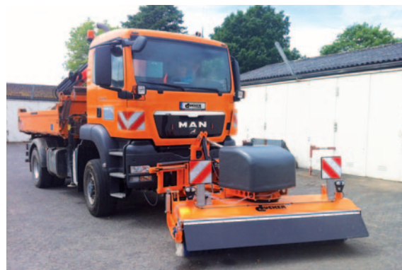
FKM sweeper, hydraulically driven by truck, with water spraying device and water tank
