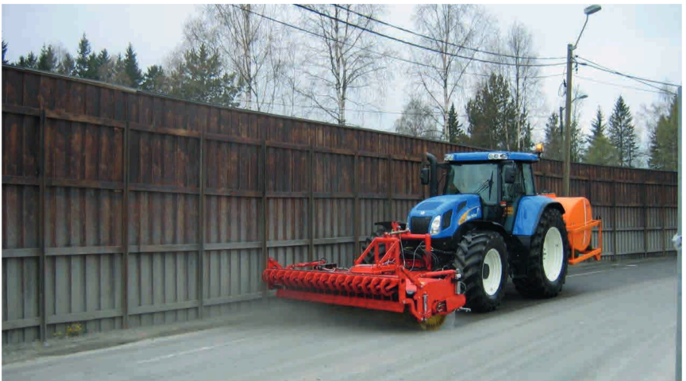
SFK sweeping machine with high-pressure system and water tank
