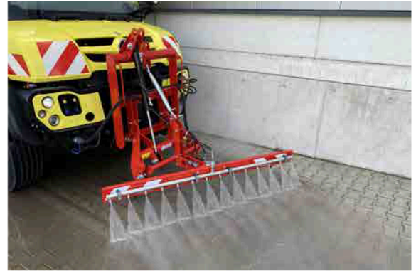
High-pressure water bar mounted on the attachment plate
