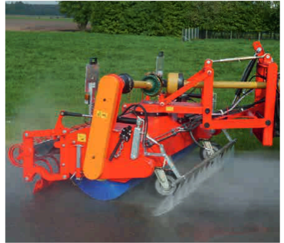
High-pressure bar mounted on sweeping machine SFK
