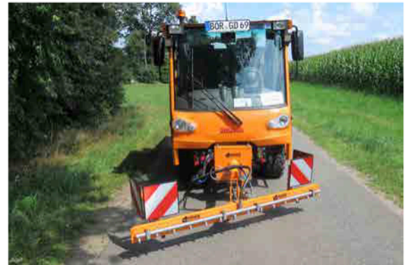
High-pressure water bar on the municipal vehicle
