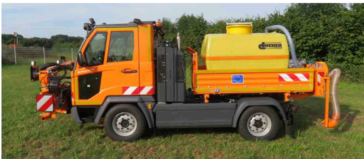
Water tank WHT 1800-PE with 1800 ltr. capacity
