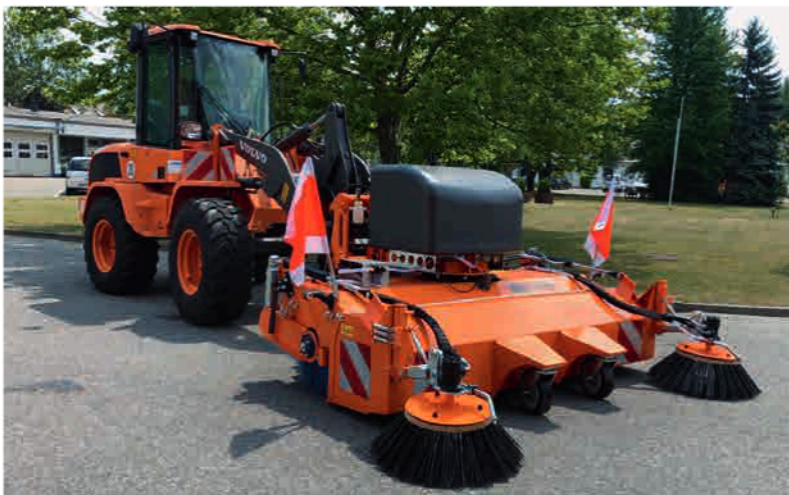
FKM sweeping machine with built-in water tank and water spraying device
