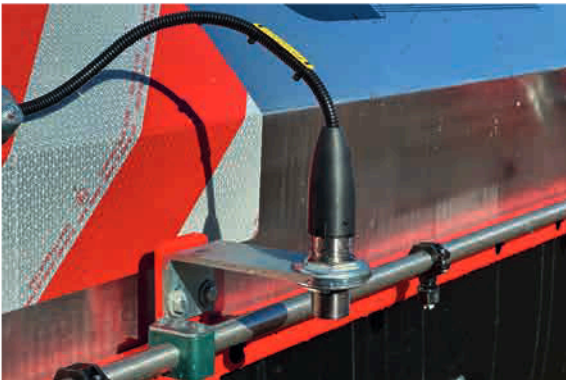
Automatic button on the tunnel washing system
