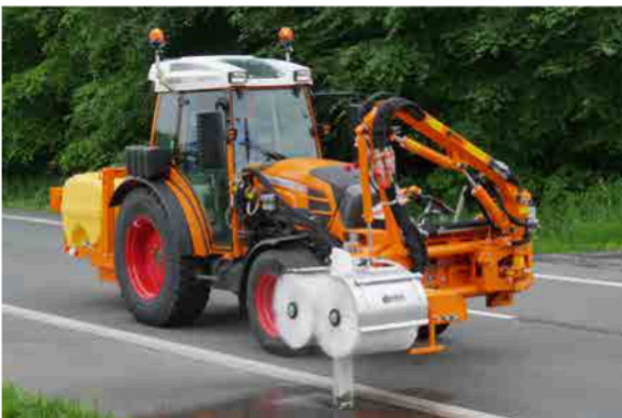
LPW 500 when cleaning delineators
