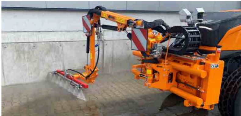
High-pressure water bar mounted on outrigger
