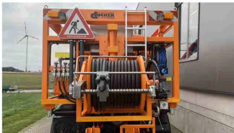
Channel flushing device on the cube frame from the water tank
