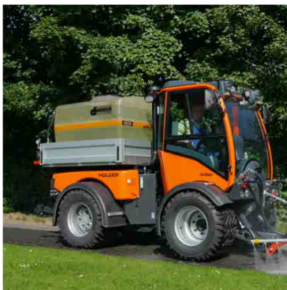
Water tank WHT 1000-GFK with 1000 ltr. capacity
