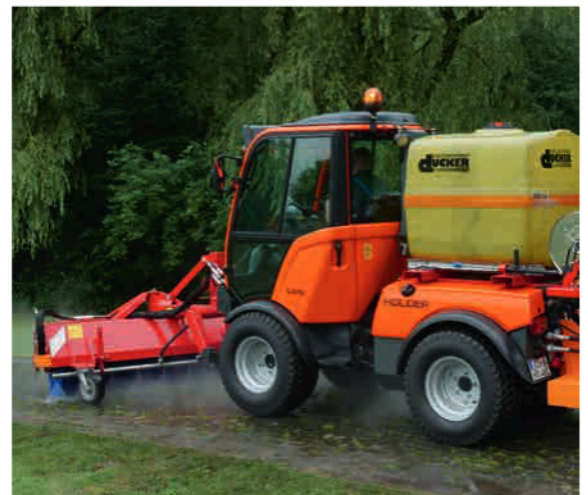
HDK sweeping machine with high-pressure bar
