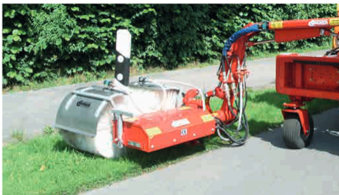
LPW 500 - Delineator and sign washing system Working width: 500 mm Rotation speed: max. 375 rpm Weight: approx. 150 kg
