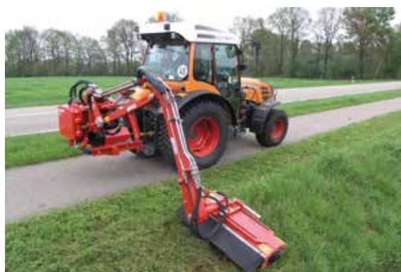
KBM 350 as rear attachment with flail mowing head
