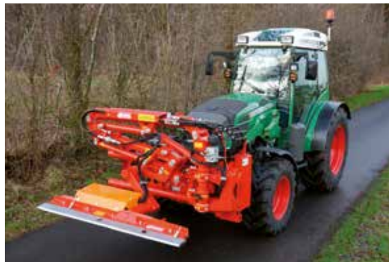
DBM 400 in transport position on Fendt tractor
