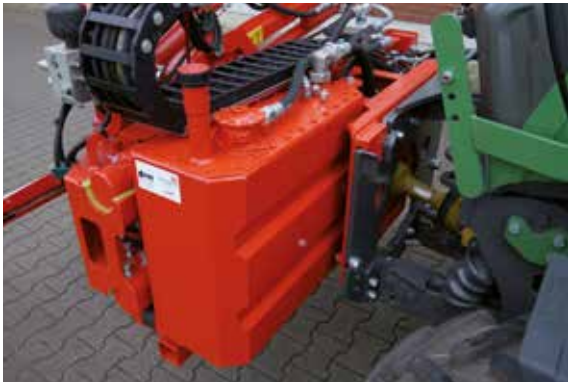
DBM 400, integrated hydraulic system
