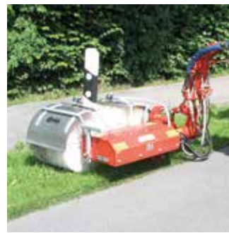
LPW 500 Reflector post- and signs-cleaner Working width: 500 mm Revolutions of shaft: 375 rpm Weight: 150 kg
