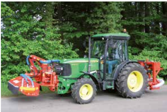
UNA 200 in transport position on John Deere tractor, divided build
