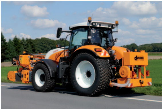
MK mower combination in divided build (hydraulic unit in rear attachment) on Steyr tractor
