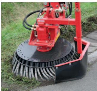
PFP 600/900 Pavement Cleaner Working width: 600/900 mm Revolutions of shaft: 150 rpm Weight: 140 kg/190 kg
