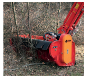
GMK 12 Brushwood-Mower-Head Working width: 1200 mm Cutting thickness: until 60 mm Revolutions of shaft: 2700 rpm Weight: 350 kg
