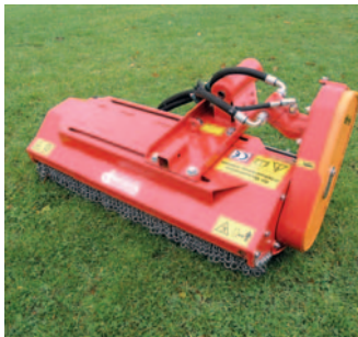
TMK 10/13 Flail-Mower-Head Working width: 1000/1300 mm Revolutions of shaft: 2200 rpm Weight: 180 kg/210 kg
