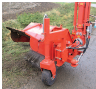
RWB 600 Radial-Weed-Brush Working width: 600 mm Revolutions of shaft: 150 rpm Weight: 320 kg
