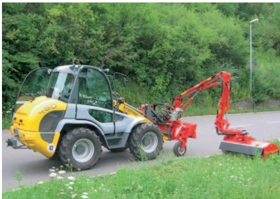
UNA 500 in action on the wheel loader
