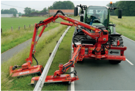
MK mower combination consisting of DUA 700 and RSM on Fendt tractors for simultaneous mowing behind and under guide devices
