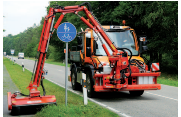
DUA 800 - The telescope arm enables the operator to run over traffic signs.
