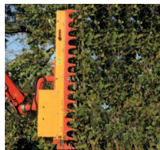
AWS 13/22 Branch- and Hedge-Cutter Working width: 1300/2200 mm Cutting thickness: until 110 mm Weight: approx. 160 kg / 230 kg
