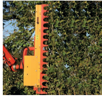
AWS 13 / 22 Branch and wall hedge cutter Working width: 1300 / 2200 mm Cutting thickness: up to 110 mm Weight: ca. 160 kg / 230 kg
