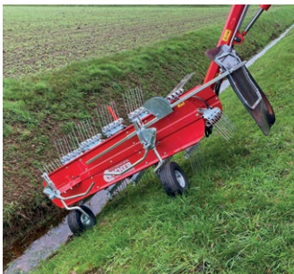
DBR 1800 / 2000 band screen Working width: 1800/2000 mm Revolutions of shaft: 450 rpm Weight: 230 / 250 kg
