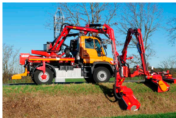
The mower combination with three mower heads enables 3 cuts to be mown in one pass
