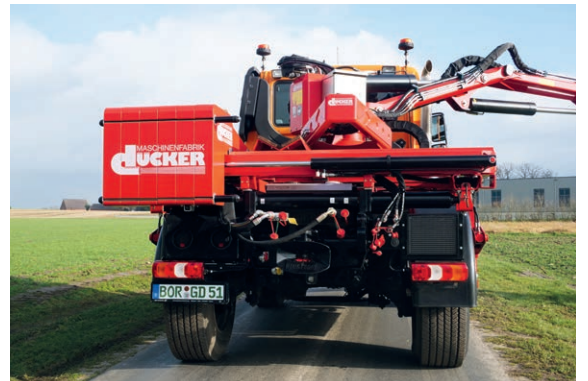
The hydraulically displaceable counterweight
