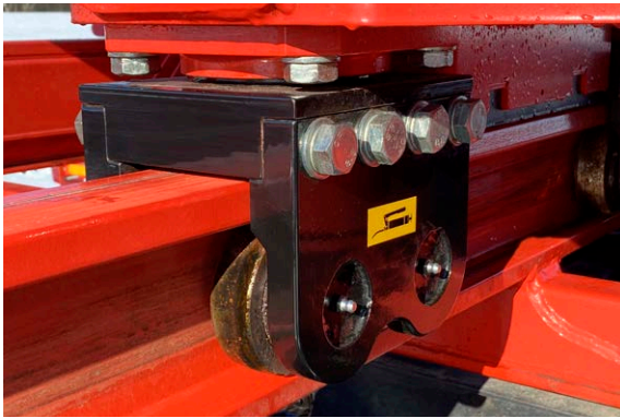
The slider can be moved on ball-bearing rollers
