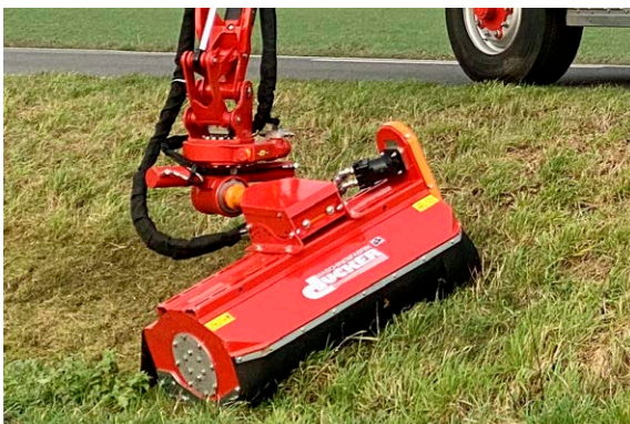
Device connection with 2-axle rotating device
