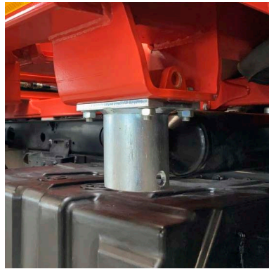
Mounting on the platform intermediate frame with tool-free locking enables easy assembly
