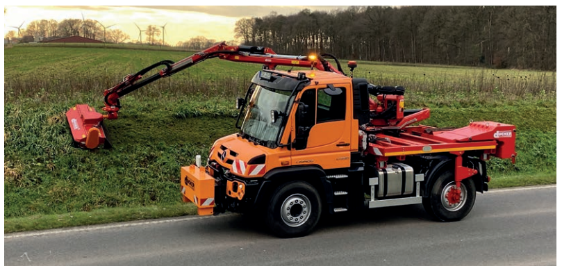
When the outrigger is swivelled backwards and forwards, the implement is automatically guided parallel to the vehicle
