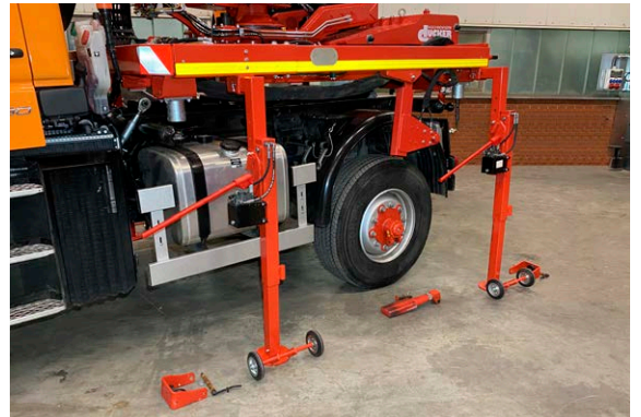
Hydraulic parking supports movable on rollers
