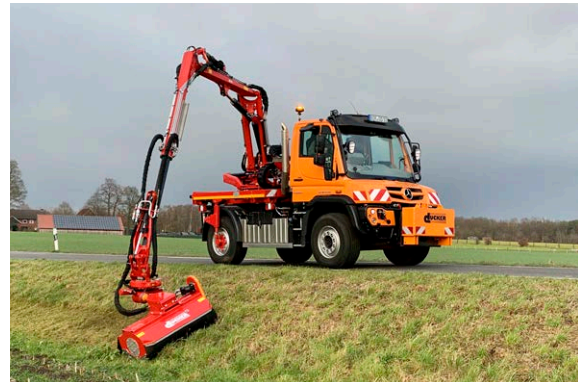
The DAM 1050 mowing a slope
