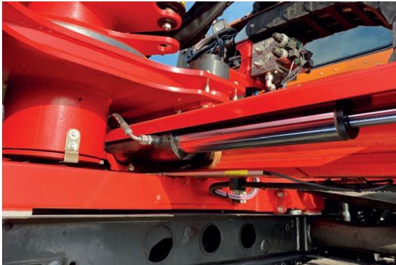
The sliding of the slider via hydraulic cylinder
