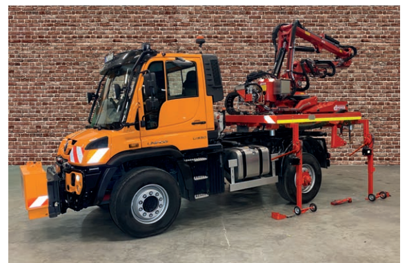
Easy dismantling of base frame and outrigger
