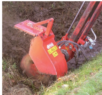
GSF 600 Ditch bottom cleaner Working width: 600 mm Revolutions of shaft: 800 rpm Weight: 230 kg
