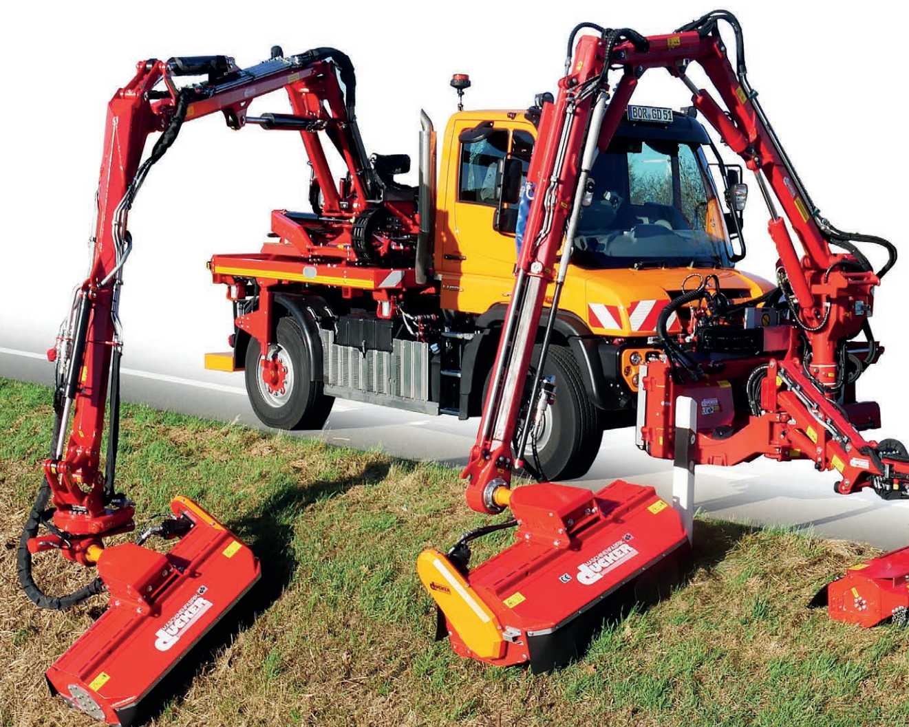
The mower combination with three mower heads enables 3 cuts to be mown in one pass
