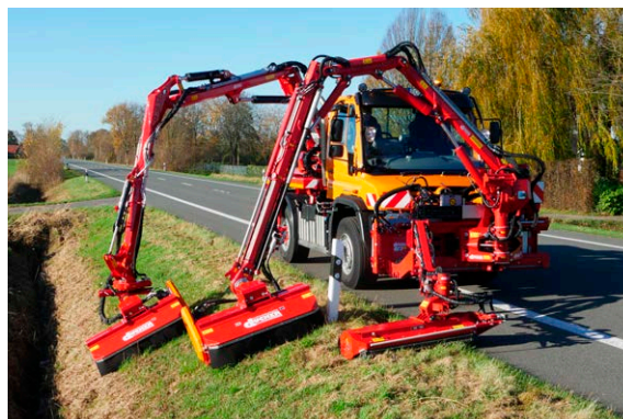
DAM top mounted outrigger in combination with the Dücker MK 25 mower combination
