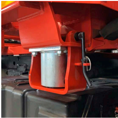
Mounting on the platform intermediate frame with tool-free locking enables easy assembly
