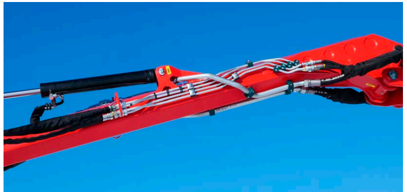
Fix laid steel hydraulic lines
